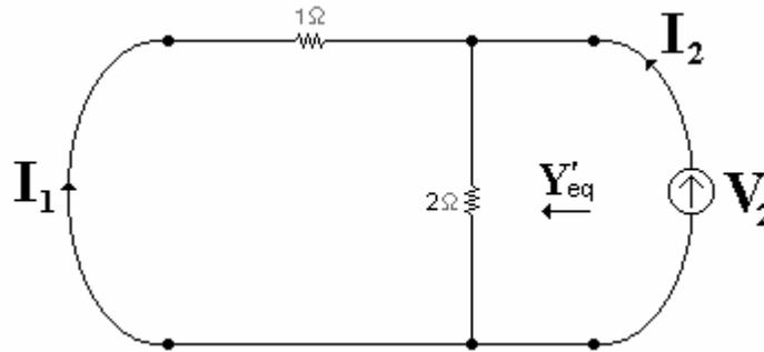
$$Y_{12} = \left. \frac{I_1}{V_2} \right|_{V_1=0} = \frac{(-1)(V_2)}{V_2} = -1 \text{ mhos}$$
