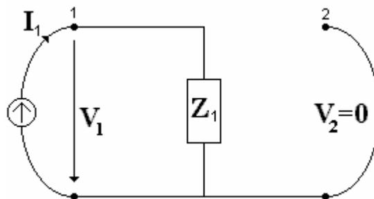
$$Y_{11} = \left. \frac{I_1}{V_1} \right|_{V_2=0} = \frac{\frac{1}{Z_1} V_1}{V_1} = \frac{1}{Z_1} \text{ mhos}$$
