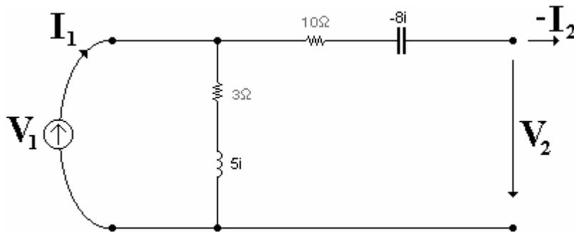
$$V_1 = (3 + 5i) I_1 = V_2$$
