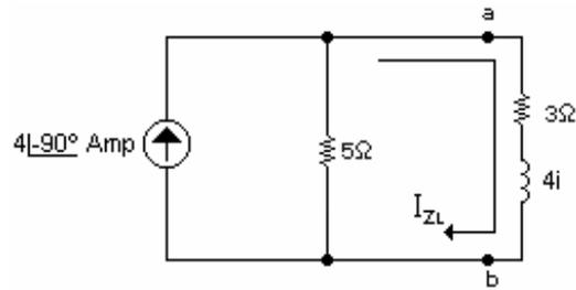
$$I_{z_L} = \frac{5(4\angle -90^\circ)}{5 + 3 + 4i} = \frac{20\angle -90^\circ}{8.94\angle 26.56^\circ} = 2.23\angle -116.56^\circ \text{ amp.}$$
