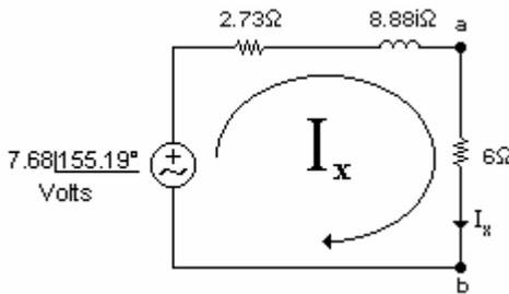
$$I_x = \frac{7.68 \angle 155.19^\circ}{8.73 + 8.88i} = 0.61 \angle 109.7^\circ \text{ amp.}$$
