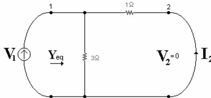
$$Y_{11} = \left. \frac{I_1}{V_1} \right|_{V_2=0} = \frac{Y_{eq}(V_1)}{V_1} = 1 + \frac{1}{3} = \frac{4}{3} \text{ mhos}$$
