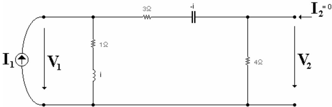
$$Z_{11} = \frac{V_1}{I_1} \Big|_{I_2=0} = \frac{(Z_{eq})I_1}{I_1} = \frac{(7-i)(1+i)}{7-i+i+1} = 1 + 0.75i$$
