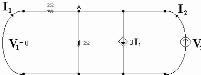
$$Y_{12} = \left. \frac{I_1}{V_2} \right|_{V_1=0} = \frac{-\left(\frac{1}{2}\right)V_2}{V_2} = -\frac{1}{2} \text{ mhos}$$
