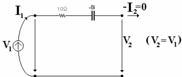
$$A = \left. \frac{V_1}{V_2} \right|_{-I_2=0} = 1$$
