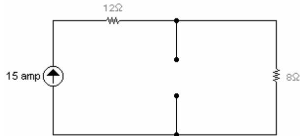
$$V_0 = (15)(8) = 120 \text{ volts}$$
