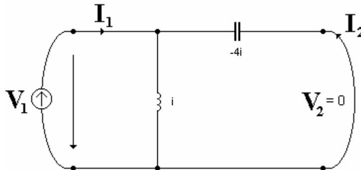
$$h_{11} = \left. \frac{V_1}{I_1} \right|_{V_2=0} = \frac{V_1}{YV_1}$$
